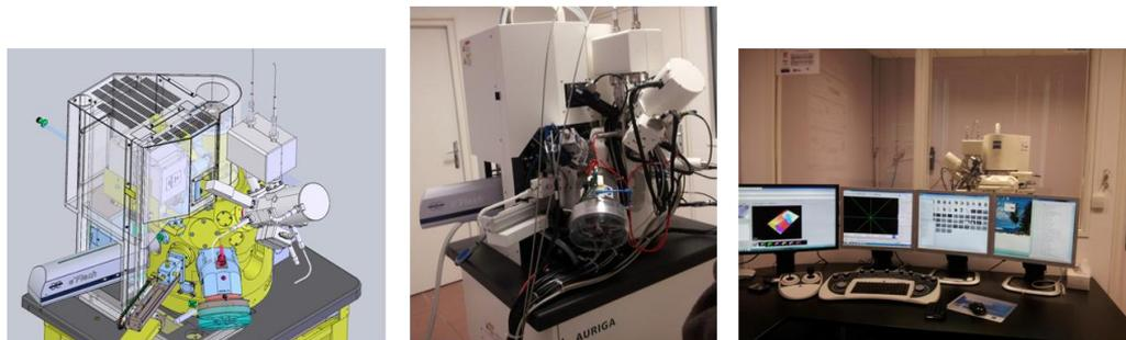
Fig. 1: Custom made AURIGA 40 – ZEISS microscope equipped with the Bruker EBSD detector, as installed at LEM3-CNRS METZ FRANCE
